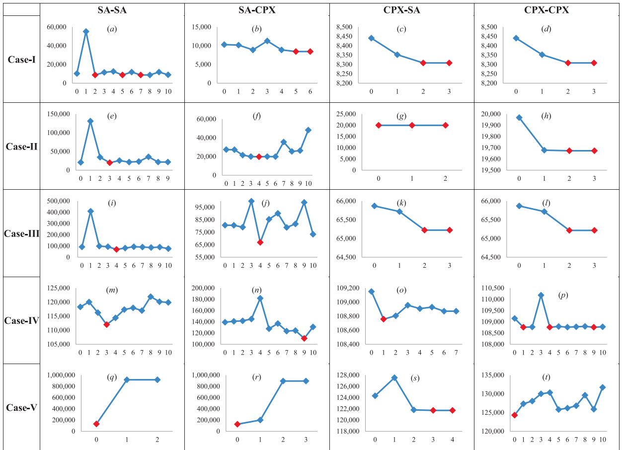
Fig. 7. Total costs in terms of iteration on tight due dates. The vertical axes show the objective value, and the horizontal axes show the number of algorithm iterations, ranging from 1 to 10 (the maximum number of iterations), where 0 denotes the initial iteration. The red markers show the minimum total costs.
